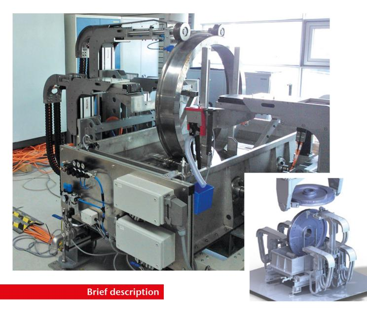
The ultrasonic test system presented here supplements the product line for rail industry with a production- based wheel testing system. Our long-term experience with various other testing systems benefits the conception and development of this wheel testing system, significantly shaping the design as an "in-line" testing system.
