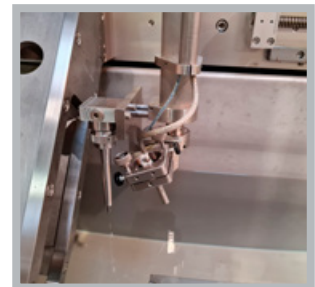
Probe holder with scribe marker
