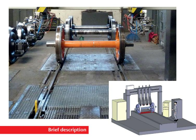
For the so-called heavy maintenance involving the removal of the wheel sets from the railway vehicle, extensive testing procedures are required to evaluate the condition of the axles on the wheel set. This process calls for the complete inspection of the axles over their entire length for operational fatigue. As long as the wheels are not pressed off, this can be performed using ultrasonic testing technology.
